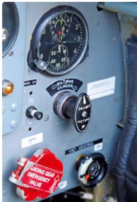
How to blow the gear down in an emergency: main air valve off, select undercarriage down, and then open the red valve
